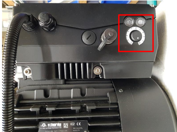
Fig. 18: Rotary control on the motor
