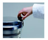
**11.** By turning the knurled knobs to the right, tighten the sieve stack evenly until the toothed belts are tightly clamped!
