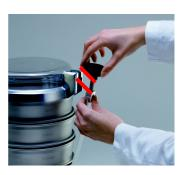
**10.** Then attach the knurled knobs to the holders of the sieve cover!
