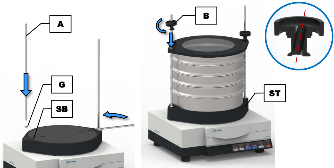
Fig. 6: Installation of the sieve clamping unit "standard"
