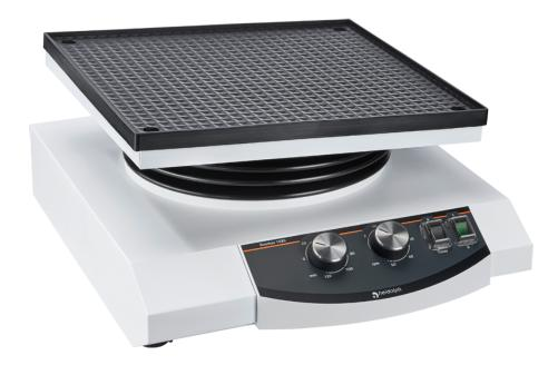
Containers are safely fixed on the anti-slip rubber mat even at high speeds. The speed is variably adjustable between 2 and 50 rpm. The shaker can be operated in continuous operation or with a timer (max. 120 minutes).
