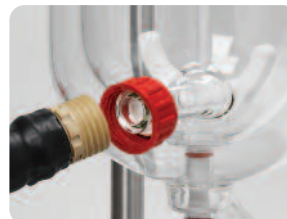
PTFE stirrer guide provides whip-free agitation
